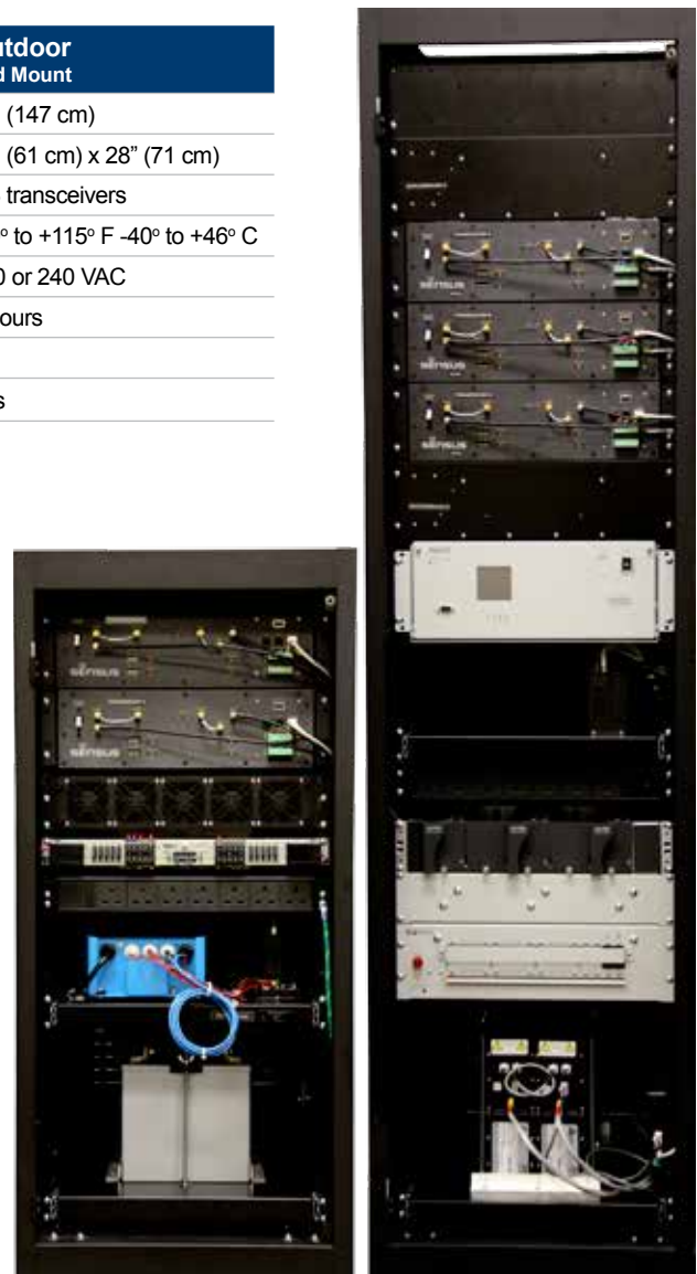
Sensus D-100 and T-100 Base Stations shown in indoor short and tall rack mount configurations.
