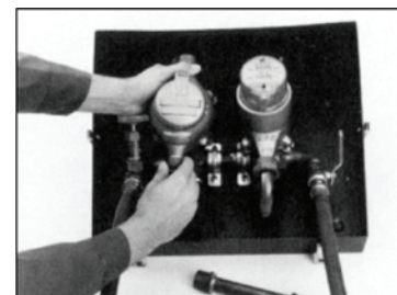
Special factory-calibrated 5/8" SR II Meter with Reset-table Electronic Register
